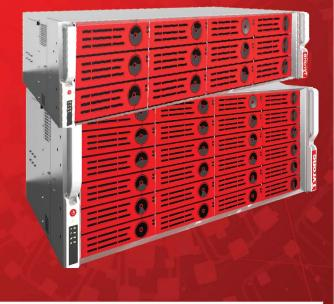
JBOD solutions from Tyrone Opslag FS2 is the perfect combination for expanding your storage needs. We have a series of JBOD to suite all kind of requirements. The hard disk box avaiable in various sizes are suitable for SAS and SATA Hard Drives. It uses the SAS controller to connect to the main box or to other JBOD. Please speak to your local product expert on suitable connectivity and other details or write to <u>support@tyronesystems.com</u>.
